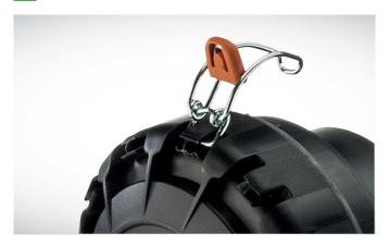
The special end caps prevent jamming of the cover and housing. Color-coded fasteners enable reliable servicing even when visibility conditions are unfavorable. In order to meet the installation space requirements, the fasteners can be positioned on the cover according to customer requirements.
