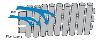
The fluid changes direction as it comes into contact with the media fibers, as illustrated above. As the fluid flows through the media, it changes direction continuously as it works its way through the maze of media fibers. As it works its way through the depths of the layers of fibers, the fluid becomes cleaner and cleaner. Generally, the thicker the media, the greater the dirt-holding capacity it has.
