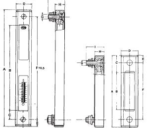
Bolt torque: 10 ft.-lbs/Nt-m. Inside nut for tightening directly on the tank. Suggested mounting hole diameter: 11mm or 13mm.
