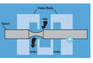
This illustration of a simple hydraulic valve illustrates how particles damage components. In normal operation, the spool slides back and forth in the valve
