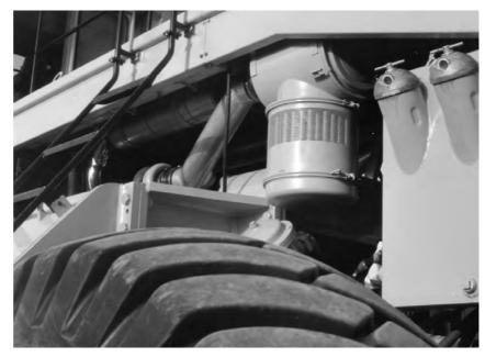
This STG Donaclone, mounted on a large mining machine, is protecting the engine from harmful dirt in this severely dusty environment.
