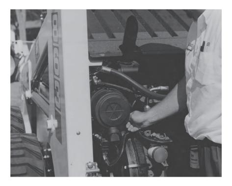
The filter inside the air cleaner is also quite different from the traditional design: one-piece molded urethane endcaps encase the ends of the media and filter liners, eliminating the metal caps and plastisol potting compound that were traditionally used. The glued-on gasket found on conventional filters is gone – now, the inside surface of the open end is actually the radial sealing surface.
