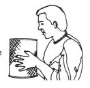
**Inspect the New Filter for Damage**
