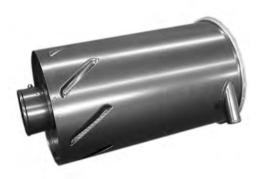
The FLB - Louvered Body Air Cleaner is a two-stage air cleaner with scavenge exhaust system and Axial Seal Sealing Technology. Body diameters in 6", 8", 10" and 12". Handles airflows of 3-17 m³/min. Sustained temperature tolerance: to 82°C.
